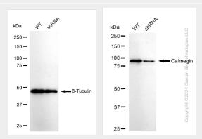
Western blotting analysis using anti-Calmegin antibody (Cat#AGI1200). Calmegin expression in wild type (WT) and Calmegin shRNA knockdown (KD) HeLa cells with 30  $\mu$ g of total cell lysates.  $\beta$ -Tubulin serves as a loading control. The blot was incubated with anti-Calmegin antibody (Cat#AGI1200, 1:10,000) and HRP-conjugated goat anti-rabbit secondary antibody respectively.
